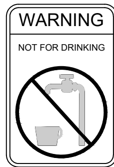
EVERY EXTERNAL SUPPLY OUTLET FROM RAINWATER RE-USE TANK TO BE LABELED WITH METALLIC WARNING SIGN
